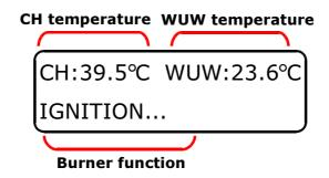
The driver may work in three working modes ("STOP", "IGNITION", "AUTOMATIC WORK"). The change of the working mode happens when the "MODE/\infty" button is pressed on the regulator's panel. Activating the "STOP" mode is possible in all modes after pressing the "MODE/\infty" button for 3 seconds. This mode activates procedures connected with the burner's putting out i.e. burning off and cleaning.
