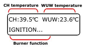
The burner may work in three working modes ("STOP", "IGNITION", "AUTOMATIC WORK"). The mode changes when the "MODE/\rightarrow" button is pressed. Activating the "STOP" mode is possible in all modes after pressing the "MODE/\rightarrow" button for 3 seconds. When Stop is activated, the burner goes at "Burning off" process (if there is fire) and the at "Cleaning" process.
